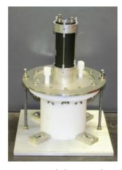
FIGURE 2: PTFE tub detector with a PMT.
