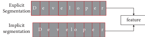
FIGURE 3: The difference between explicit segmentation and implicit segmentation.
