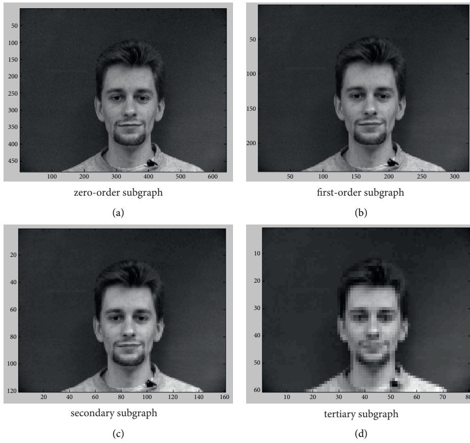
FIGURE 4: Pyramid subgraph obtained by wavelet decomposition. (a) Zero-order subgraph. (b) First-order subgraph. (c) Secondary subgraph. (d) Tertiary subgraph.
