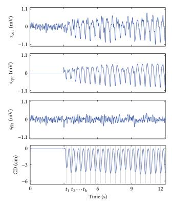
FIGURE 2: Filtering example of a 12-s segment. In the first 3 s there is no artifact and the underlying VF is visible. The filter estimates the artifact,  $s_{\rm cpr}$ , using information derived from the CC marks, indicated by vertical lines in CD ( $t_k$  instants).
