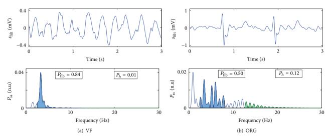
FIGURE 5: Example of the frequency domain analysis for VF (a) and an ORG (b) window. VF concentrates most of its power around the fibrillation band (blue). ORG rhythms have a spectrum with many harmonics of the heart rate and thus larger  $P_h$  (in green).
