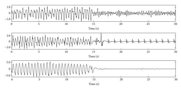
FIGURE 1: ECG segments in mV recorded in patients in OHCA. The top panel shows a VF, the middle panel shows a PEA, and the bottom panel shows an asystole. In all cases CPR artifacts corrupt the ECG in the initial 15 s interval. In the second 15 s interval chest compressions were stopped and the ECG shows the underlying rhythm.
