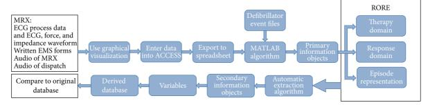
FIGURE 2: The process of deriving the variables from the manual review; the generation of the representations used for the further algorithmic reasoning for deriving the variables automatically.
