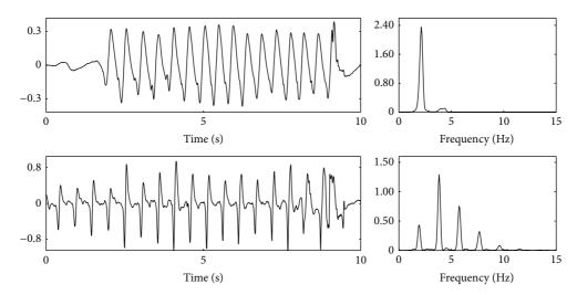
FIGURE 2: Two examples in the time and frequency domain of CPR artifacts recorded in OHCA patients in asystole. The figures show the ECG in mV and the normalized power spectral density (PSD) in the frequency domain. The first example has pauses in chest compressions, a rate of 133 cpm (2.22 Hz), and small harmonic content. The second example has no pauses, a rate of 116 cpm (1.93 Hz), and large harmonic content.
