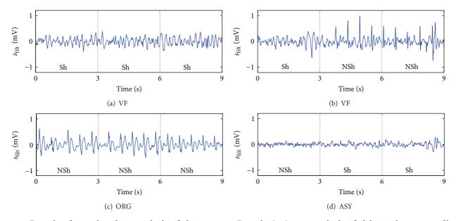
FIGURE 7: Examples of correctly and incorrectly classified 9 s segments. Examples (a, c) are correctly classified despite the presence of large filtering residuals. However, in the VF of panel (b) spiky filtering artifacts cause the erroneous classification. In the ASY of panel (d) filtering residuals are large in the last two windows causing the shock diagnosis.
