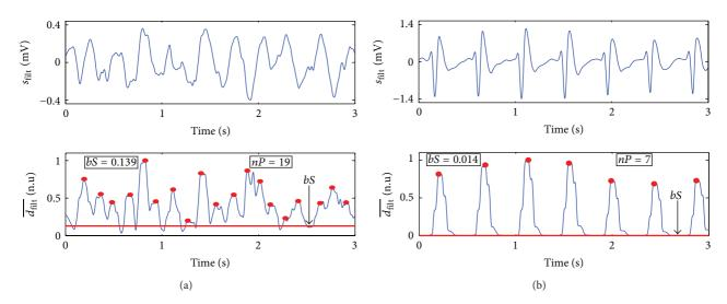
FIGURE 4: Example of the slope analysis for VF (a) and an ORG (b) window. During VF the slope,  $\overline{d_{\text{filt}}}$ , is irregular with many peaks, whereas ORG rhythms are regular with fewer peaks and concentrate most  $\overline{d_{\text{filt}}}$  values around the baseline.
