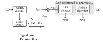
FIGURE 1: Block diagram of the new approach to rhythm analysis during CPR in which an adaptive filter (LMS filter based on the CD signal) is used in combination with a SAA designed to optimally classify the filtered signal,  $s_{\rm filt}$ .
