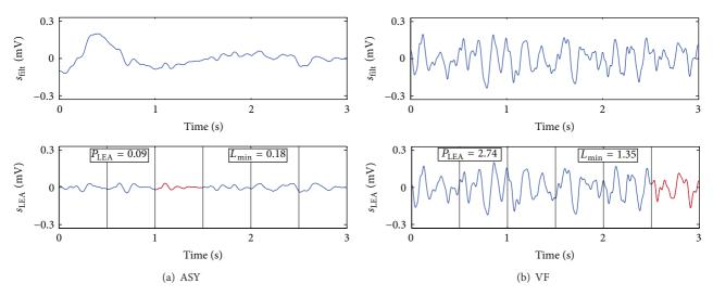
FIGURE 3: Examples of a LEA rhythm (a) and a VF (b) window after filtering the CC artifact,  $s_{filt}$ , and preprocessed to suppress components under 2.5 Hz,  $s_{LEA}$ . Vertical lines separate the 0.5 subintervals, and the one with lowest activity ( $L_{min}$ ) is shown in red.
