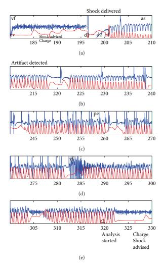
FIGURE 3: Case recording from MRX defibrillator. The blue tracing is the ECG. Impedance tracing is shown in red. The defibrillator log events (shock advised, charge, shock delivered, analysis started, and artifact detected), the rhythm transitions (vf: ventricular fibrillation, as: asystole, and pe: pulseless electrical activity), and annotations for start and end of compressions (c1 and c2) and defibrillations (d1 and d2) are shown. Refer to Figure 4 for the corresponding RORE representation.
