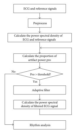
FIGURE 3: Flowchart of the enhanced adaptive filtering method.
