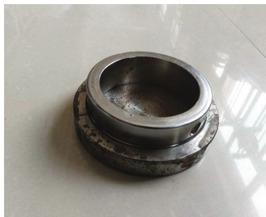
FIGURE 3: The standard penetration mold.
