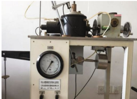
FIGURE 2: FDJ-20 direct shear apparatus.
