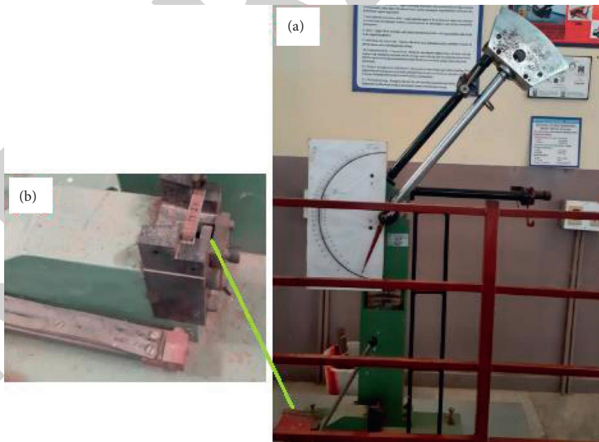
FIGURE 6: (a) Impact testing machine. (b) Izod test arrangement.
