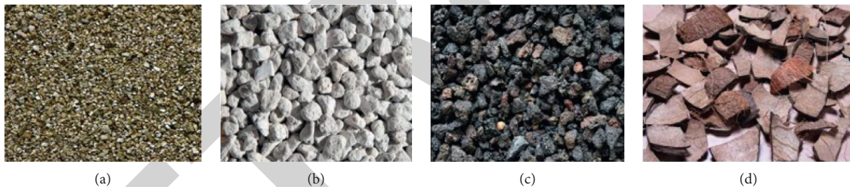
FIGURE 1: Images of lightweight aggregates. (a) Vermiculite. (b) Pumice. (c) Volcanic rock. (d) Coconut shell.
