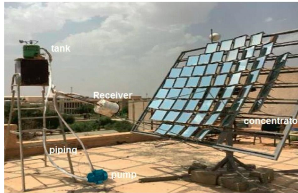
FIGURE 6: Solar dish component system.
