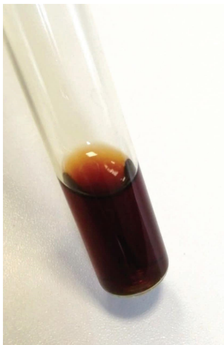
FIGURE 4: The result of the reaction with the detection of HCAs with an extract from the leaves of females of A. arguta .
