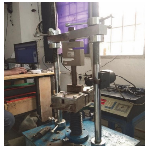
FIGURE 6: Interlaminar shear test setup.
