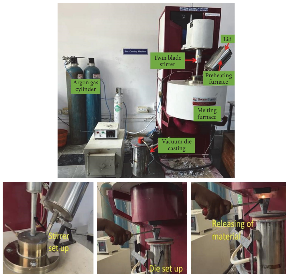
FIGURE 1: Stir-casting set up.
