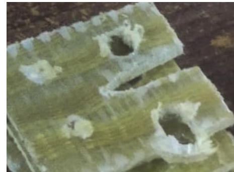
FIGURE 19: A test specimen undergone Mode-1 fracture test.
