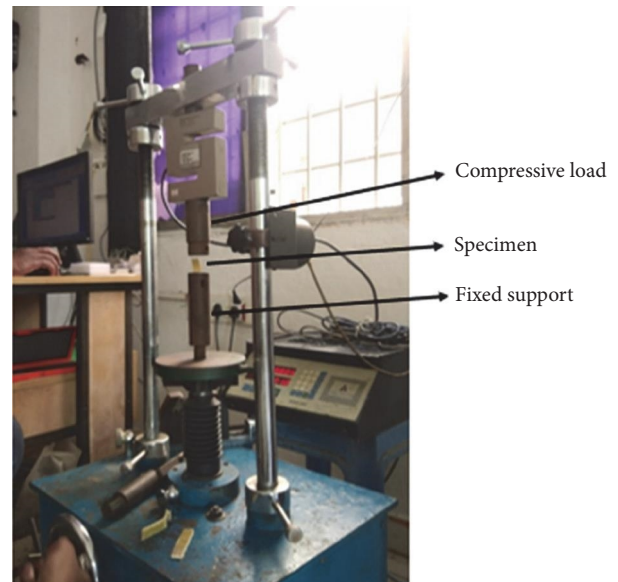
FIGURE 5: Compression test setup.
