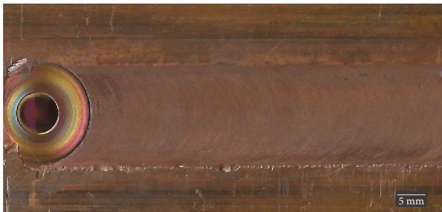
FIGURE 3: Surface appearance of fabricated Cu/ZrO 2 surface composite.
