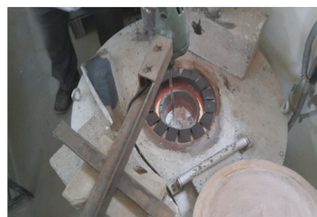
FIGURE 2: Molten metal is stirred in the furnace.
