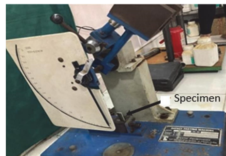
FIGURE 7: Izod impact test setup.
