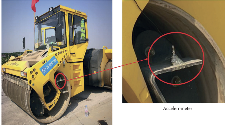
FIGURE 1: Accelerometer-equipped vibratory roller during compaction.
