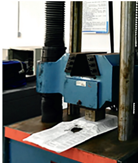
FIGURE 2: Compressive strength test of cement concrete used in this paper.
