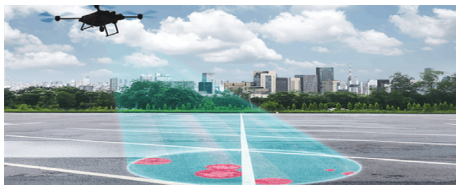
FIGURE 7: Crack detection with drone software [48].
