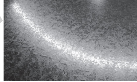
FIGURE 1: Machining workpiece surface (200 \times ). v = 280 m/min, f = 0.08 mm/r, and a_p = 0.2 mm.
