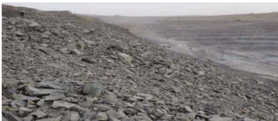
FIGURE 7: Rock fragmentation at the crest of high-bench blasting.
