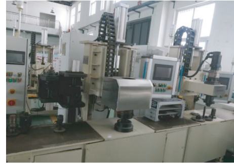
FIGURE 4: Automobile differential assembly stations.
