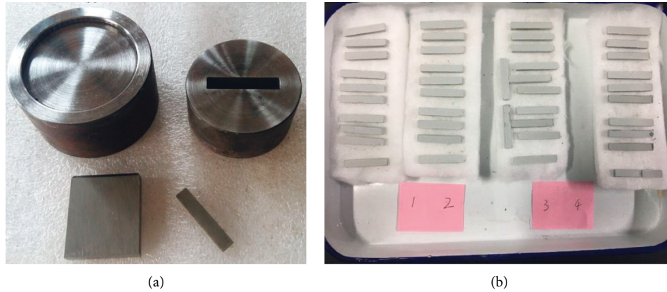
FIGURE 6: Pressing mould and green compacts of samples. (a) The special mould (b) Green compacts of SiC/Al 2 O 3 composites.
