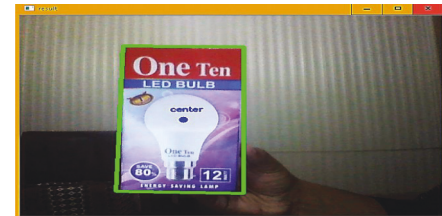
FIGURE 13: Object detection using SIFT after center point calculation.
