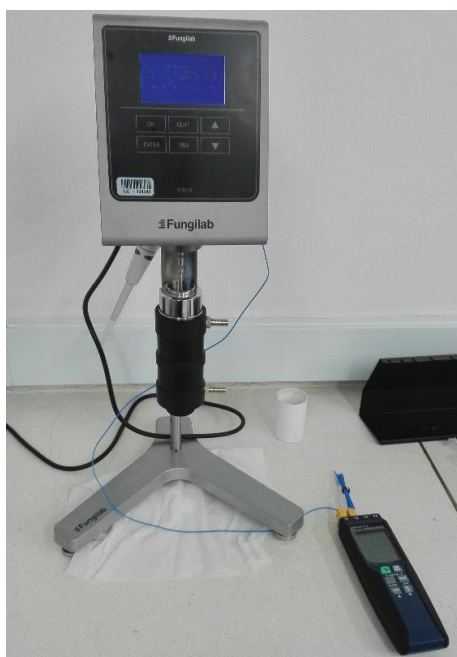
FIGURE 6: Viscometer for the reference (Fungilab Smart).
