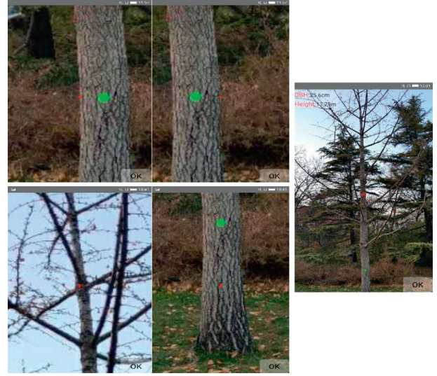
FIGURE 4: Software interface of tree height and DBH measurement.
