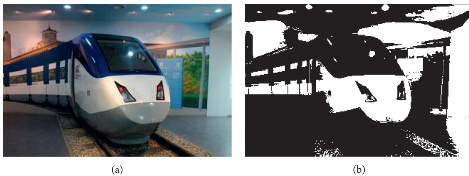
FIGURE 3: Binary processing: (a) original image and (b) binarized image.
