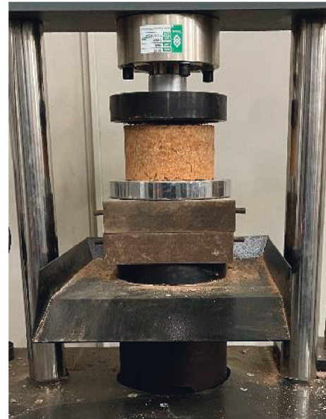
FIGURE 4: Uniaxial compression test instrument.
