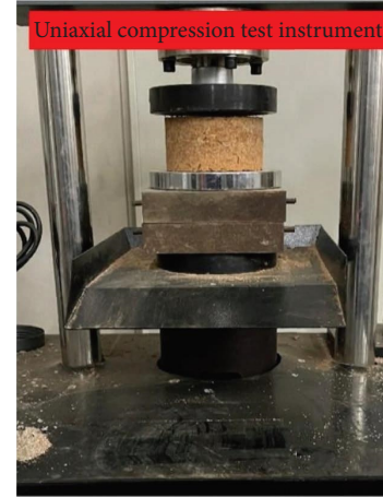
FIGURE 4: uniaxial compression test instrument.
