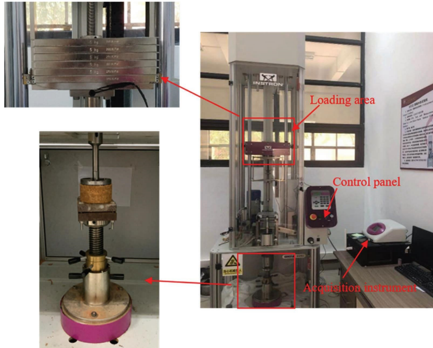
FIGURE 5: drop-weight tester.
