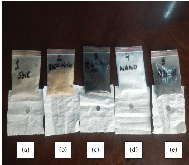
FIGURE 3: Palettes for the FTIR tests, i.e., (a) soil, (b) rice husk, (c) rice husk ash, (d) nanosilica, and (e) optimum blend of (a), (c), &amp; (d).
