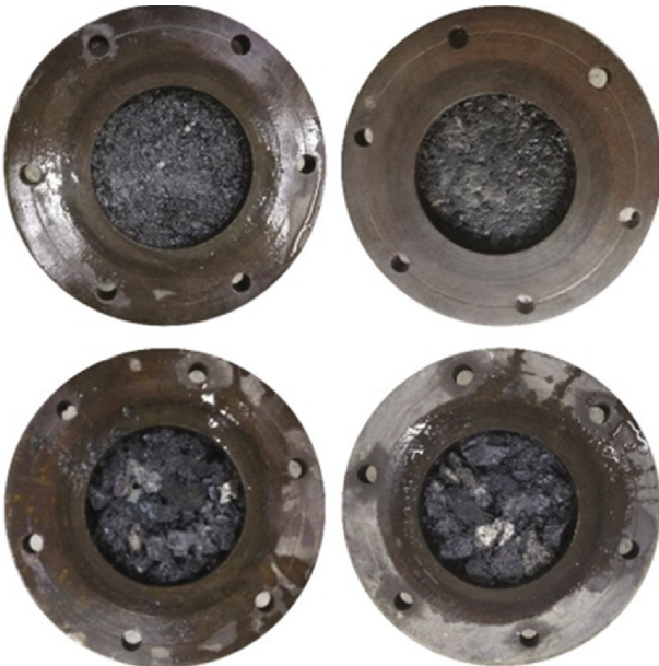
FIGURE 11: Pictures after the seepage in different sizes of gangues.
