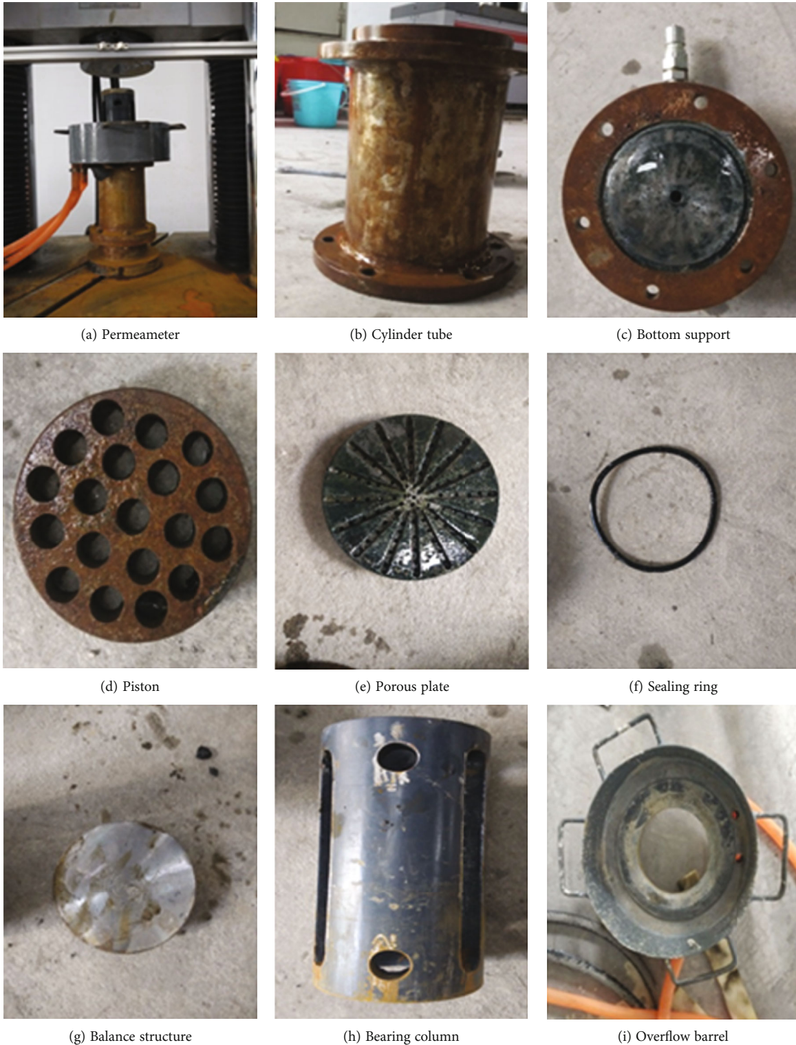
FIGURE 3: Picture of the experimental seepage system.
