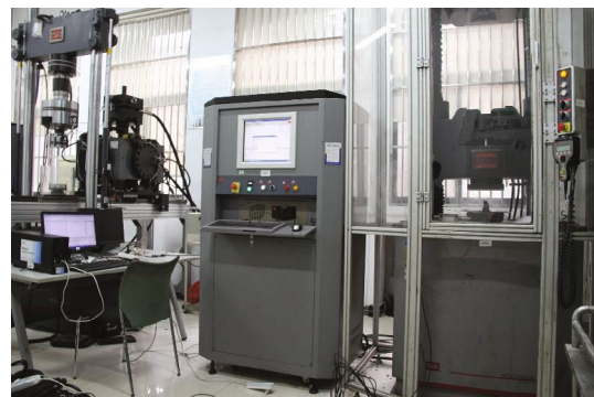
FIGURE 4: Experimental system for determining rock mechanical properties.
