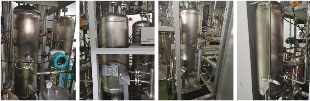
FIGURE 4: Primary and secondary separators.
