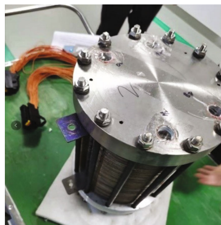
FIGURE 7: The PEM electrolyser used in the experiment.
