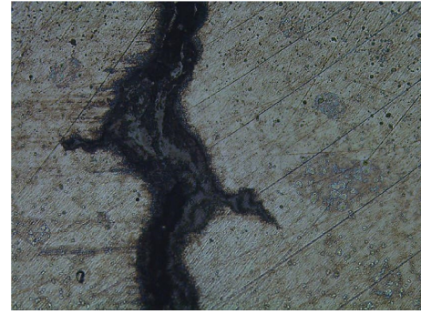
FIGURE 4: Metallographic diagram of the first layer crack of weld (200 times).
