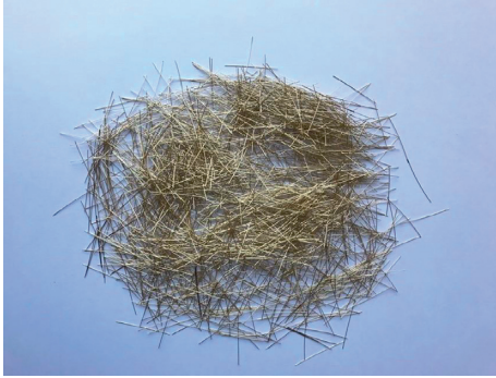
FIGURE 1: Steel fiber used for the HSFRC mixture (HF120).
