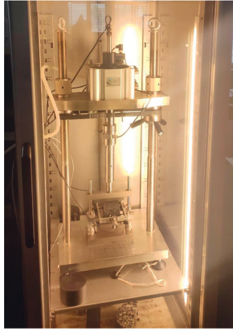
FIGURE 4: Resilient modulus test set-up.
