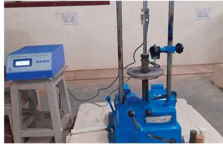
FIGURE 5: UCS test setup.
