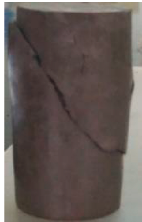
FIGURE 9: UCS failure of 2% waste plastic stabilized black cotton soil.
