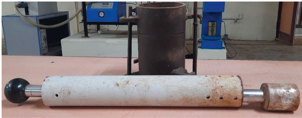
FIGURE 3: Set up for performing standard compaction tests.
