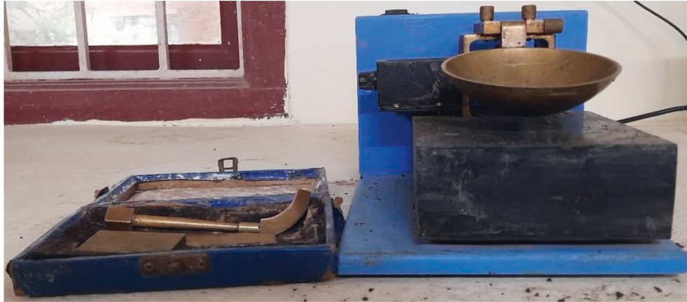
FIGURE 2: Casagrande cup for performing Atterberg limits.
