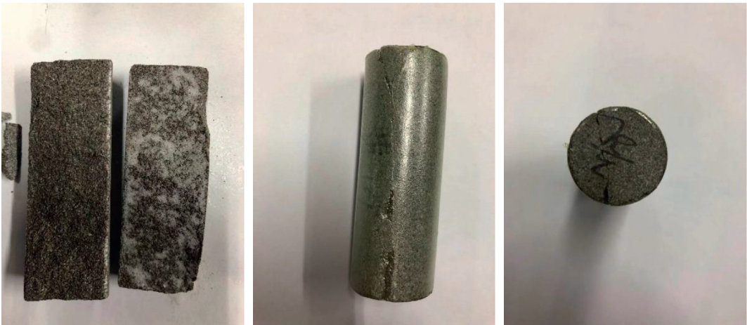
FIGURE 2: Artificial fractured core.
