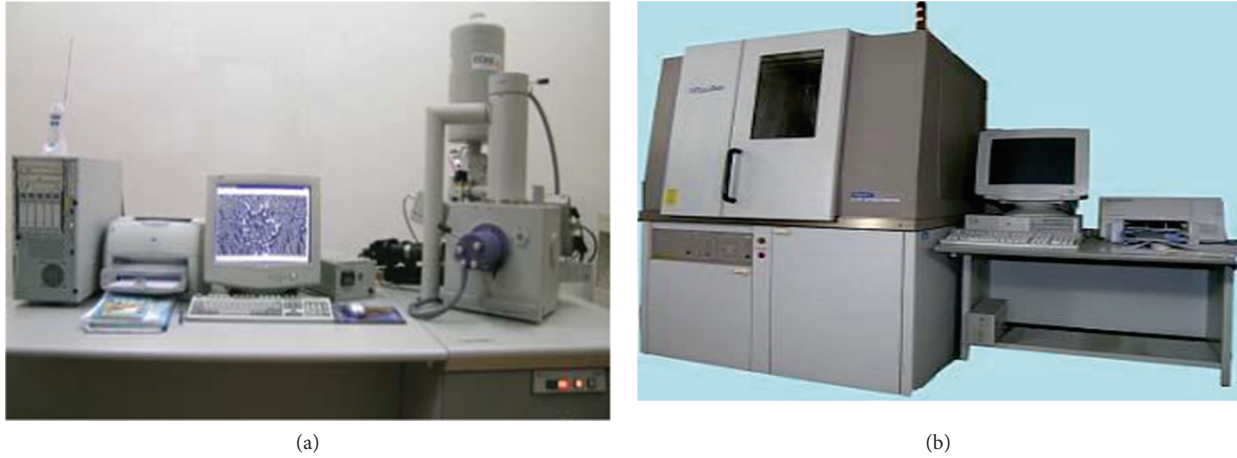
FIGURE 1: Morphology and phase test. (a) SEM. (b) XRD.
