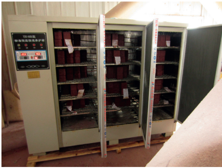
FIGURE 2: Curing of constant temperature and humidity test block for filling body.
