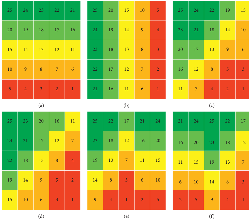
FIGURE 3: Mining sequence schemes 1–6. (a) Scheme 1. (b) Scheme 2. (c) Scheme 3. (d) Scheme 4. (e) Scheme 5. (f) Scheme 6.
