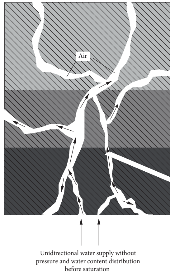
FIGURE 9: Sketch of water migration and water content distribution before saturation in Test II.
