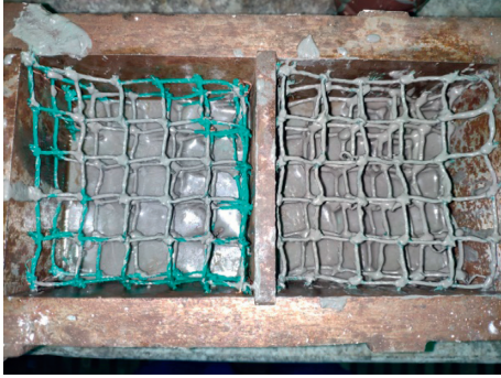
FIGURE 1: 3D flexible grid reinforcement of filling body.
