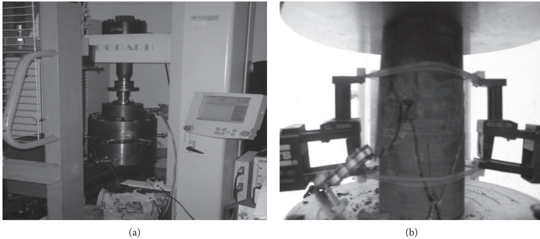
FIGURE 2: (a) Servo experimental equipment. (b) Typical uniaxial compression failure mode of rock samples.
