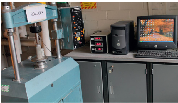
FIGURE 2: Experimental setup for unconfined compressive strength tests.
