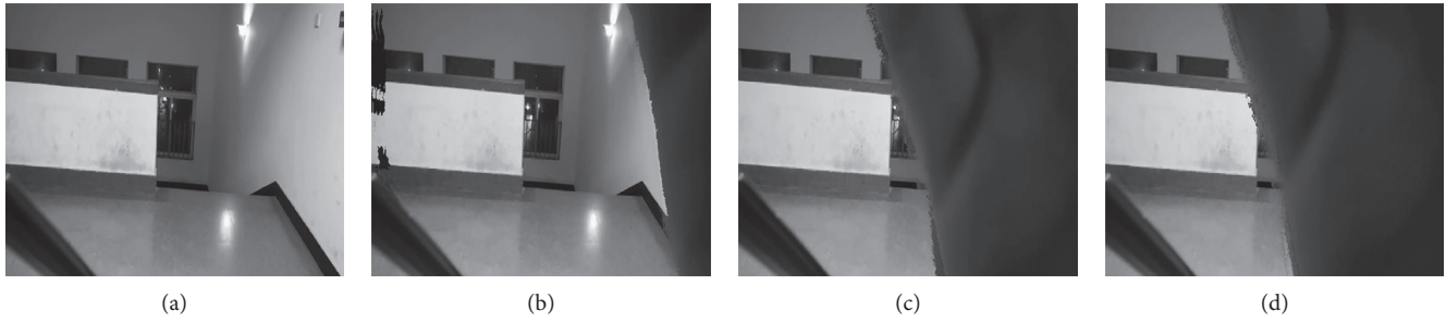
FIGURE 6: When the size of the window is 3 \times 3 , the similarity of the background image with different occluded areas and the reference image. (a) No area occluded 0.14. (b) A small area occluded 0.34. (c) A large area occluded 1.70. (d) A large area occluded 1.83.
