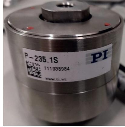
FIGURE 3: PZT model is P235.1S. (a) PZT structure dimension drawing. (b) The picture of the PZT.
