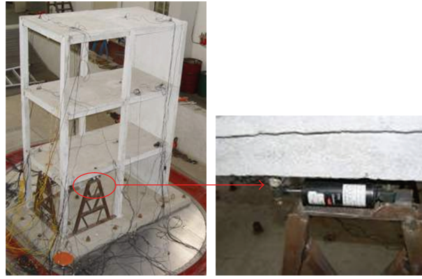
Figure 27: Eccentric vibration control experiment with MR damper.
