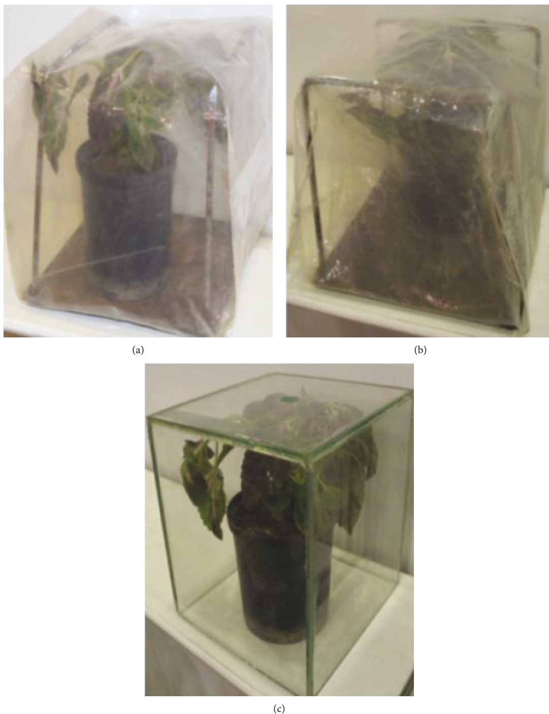
FIGURE 8: Three greenhouses: (a) LDPE without mixing, (b) LDPE mixed with 2.5 wt% \text{SiO}_2 , and (c) silica glass. This figure was reproduced from Alghdeir et al. [9] (under the Creative Commons Attribution License/public domain).
