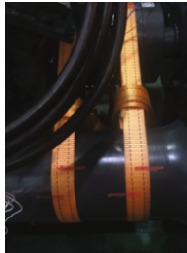
(b) The drive end is fixed by the strap
