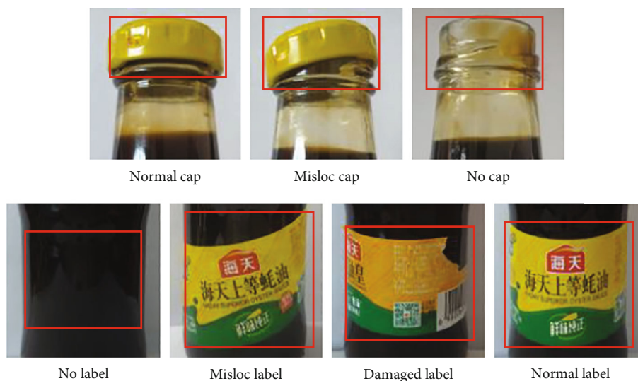
FIGURE 7: Sample of the packaging bottle defect dataset; the red frame is the ground-truth box.
