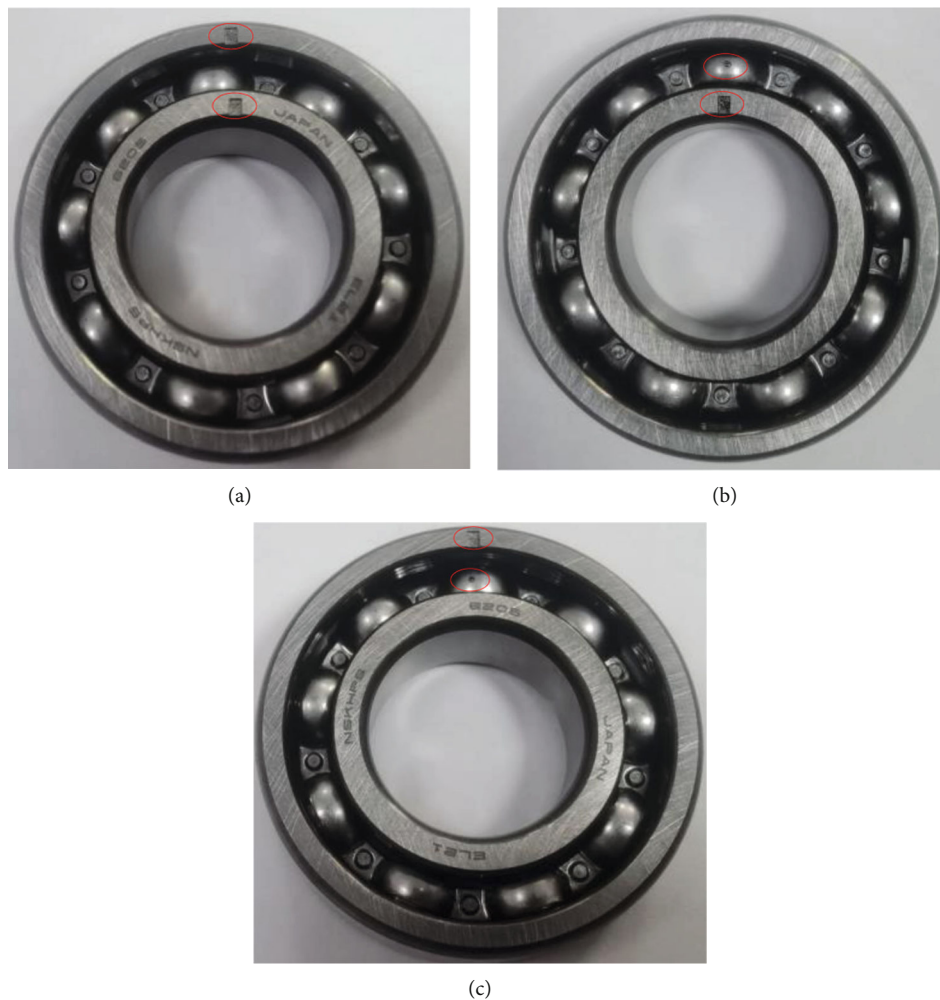
FIGURE 6: Finished fault bearings: (a) inner ring and outer ring; (b) inner ring and rolling element; (c) outer ring and rolling element.
