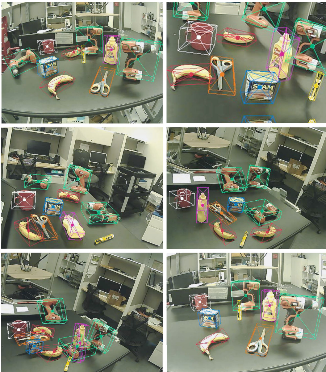
FIGURE 7: Real-world performance of the perception network in difficult backgrounds operating on seven different objects.
