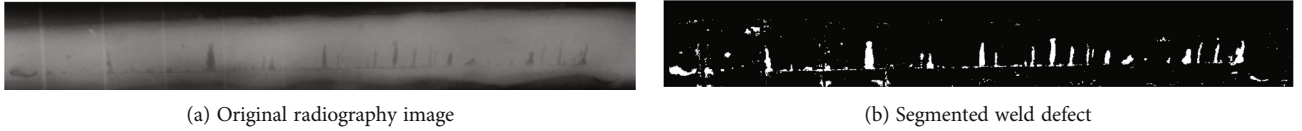
FIGURE 4: The example of weld defect segmentation.
