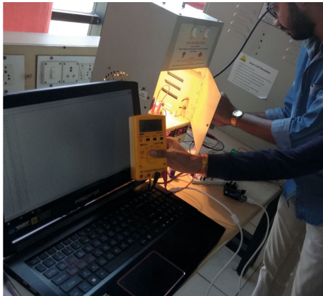
FIGURE 7: Testing datalogger with solar PV emulator.
