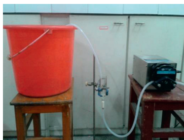
FIGURE 1: Sample collection device [41] (the left picture is the device used in the lab by authors).
