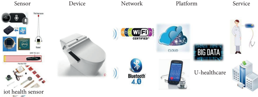
FIGURE 1: Smart health-monitoring bidet end-to-end architecture.
