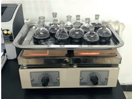
FIGURE 2: True density test process setup of the coal samples with different sulfur contents before and after the increase of the oxidation temperature.
