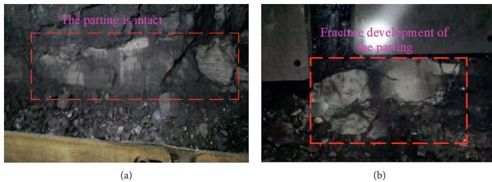
FIGURE 15: The parting before and after fracturing at the working face. (a) Before fracturing. (b) After fracturing.
