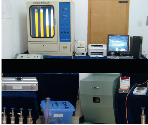
FIGURE 5: Coal seam gas content measurement instrument.
