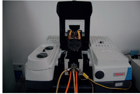
FIGURE 10: Fourier transform infrared spectroscopy in situ testing system equipped with a smart diffuse reflectance accessory.
