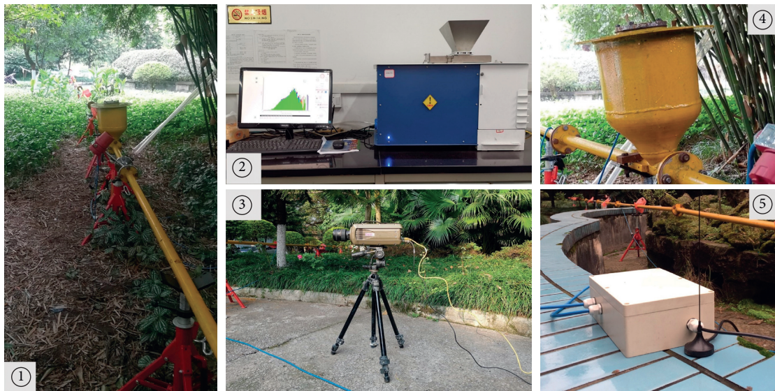
FIGURE 1: The experimental system. (a) Schematic diagram of the experimental system. (b) Physical map of the experimental system: ① Conveying pipeline. ② Particle analyzer. ③ High-speed camera. ④ Bunker. ⑤ Concentrator.
