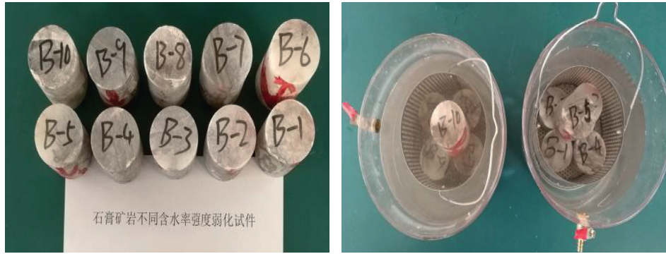
FIGURE 7: Water immersion test of gypsum rock specimens.
