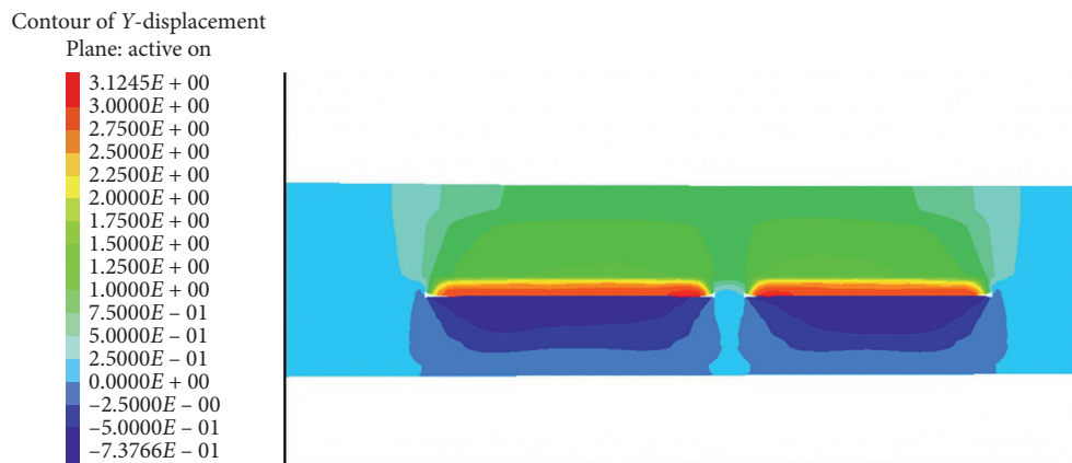
FIGURE 5: Overlaying strata subsidence of A-A cross section after 2071P is mined out.
