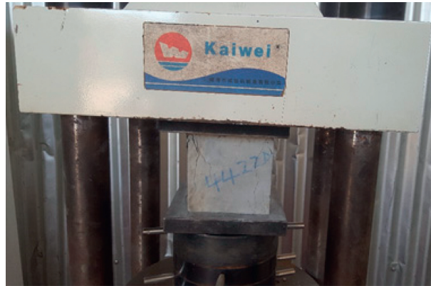
FIGURE 4: Compressive strength test setup.
