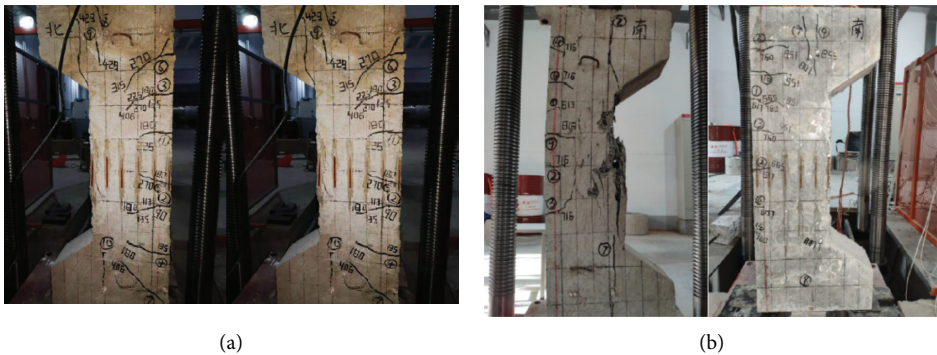
FIGURE 6: Failure mode of the specimen. (a) Large eccentric compression failure. (b) Small eccentric compression failure.
