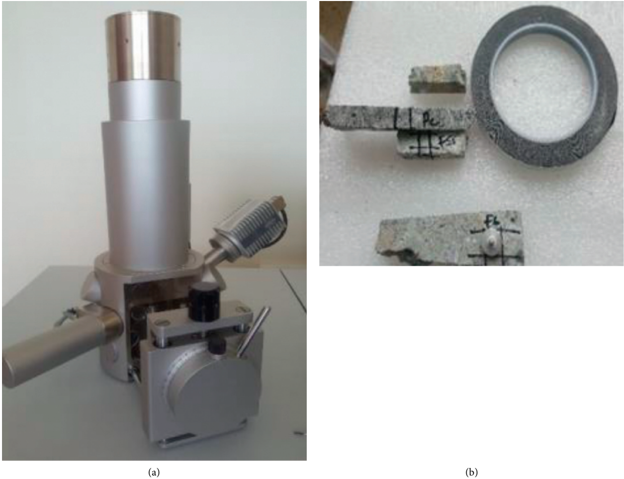
FIGURE 7: Microscopic morphology testing using a scanning electron microscope. (a) Variable SEM equipment. (b) Sample preparation for SEM.
