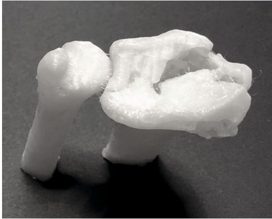
FIGURE 1: In-house printed fracture model using an FFF consumer-level desktop 3D printer (MakerBot Replicator+, MakerBot Brooklyn, New York City, New York, USA).
