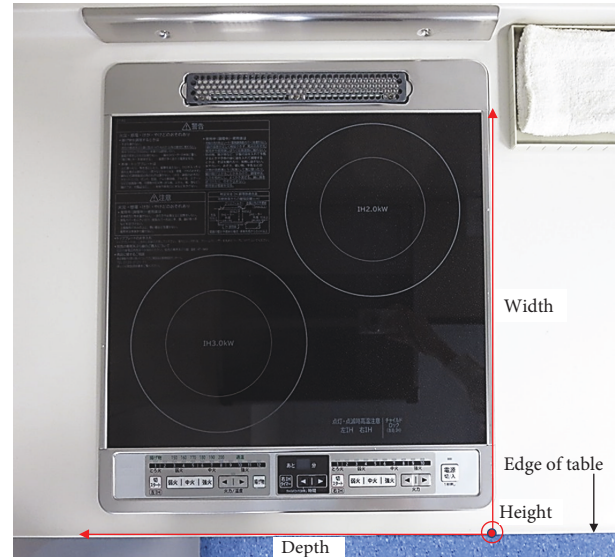
FIGURE 6: Setting of the coordinate system of IH cooking heater-1.
