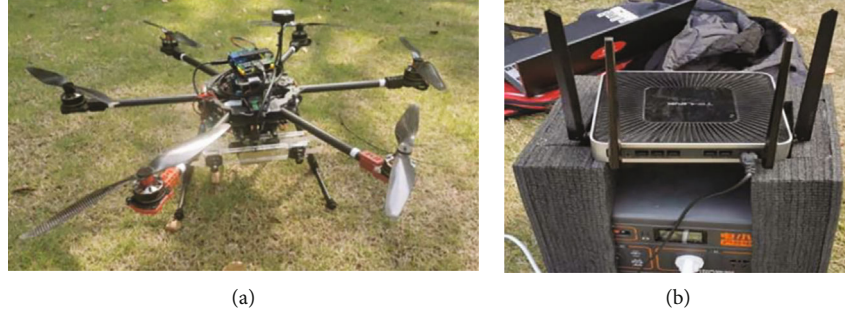
FIGURE 7: The proposed UAV system: (a) the assembled UAV; (b) the ground MEC system.
