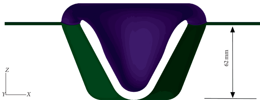
FIGURE 4: Location diagram of die parting line.
