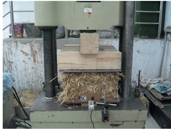
FIGURE 4: Setup and displacement sensors.
