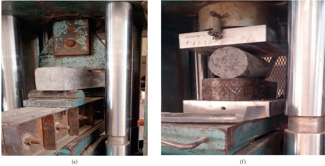
FIGURE 3: Experimental setup of concrete testing. (a) Slump test. (b) Water absorption test setup. (c) Water curing tank. (d) Compressive strength test. (e) Flexural strength test. (f) Splitting tensile strength test.
