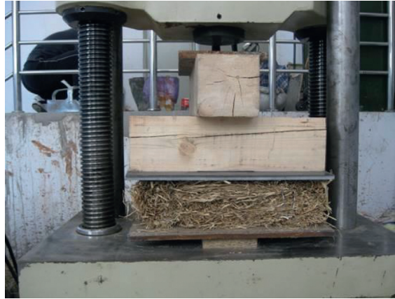
FIGURE 7: The large deformation of straw bale.
