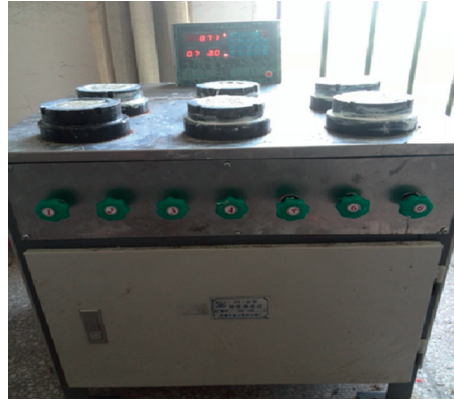
FIGURE 4: Antipenetrability performance test of sisal fiber rice husk mortar.
