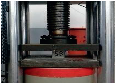
FIGURE 1: Compression test of sisal fiber husk mortar.
