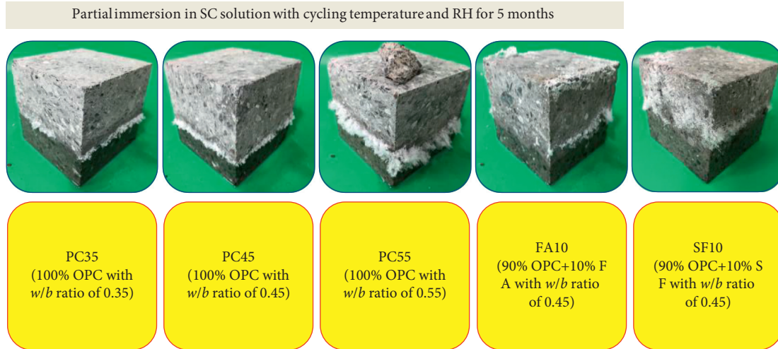
FIGURE 6: Visual appearance of various shotcrete specimens partially immersed in SC solutions subjected to cycles of temperature and RH for 5 months.
