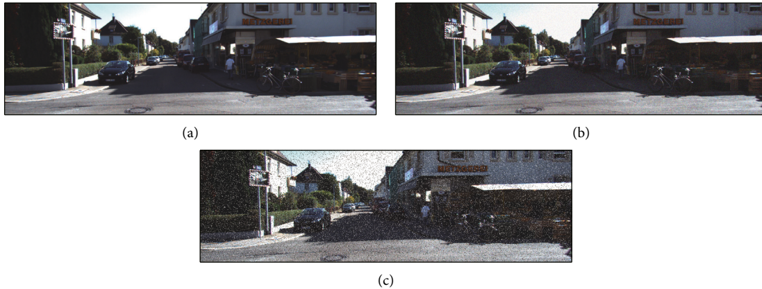
FIGURE 3: Comparison of the example scene before and after adding noise. (a) The original image. (b) The image after adding Gaussian noise. (c) The image after adding Salt-and-Pepper noise. Note that the effect of the added noise is noticeable.
