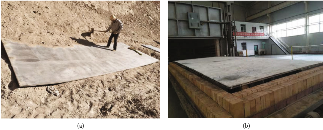
FIGURE 2: Photographs of the R60702-Gr70 clad plate after (a) explosive welding and (b) flattening (plate size: 3/25 \times 2330 \times 6000 mm).
