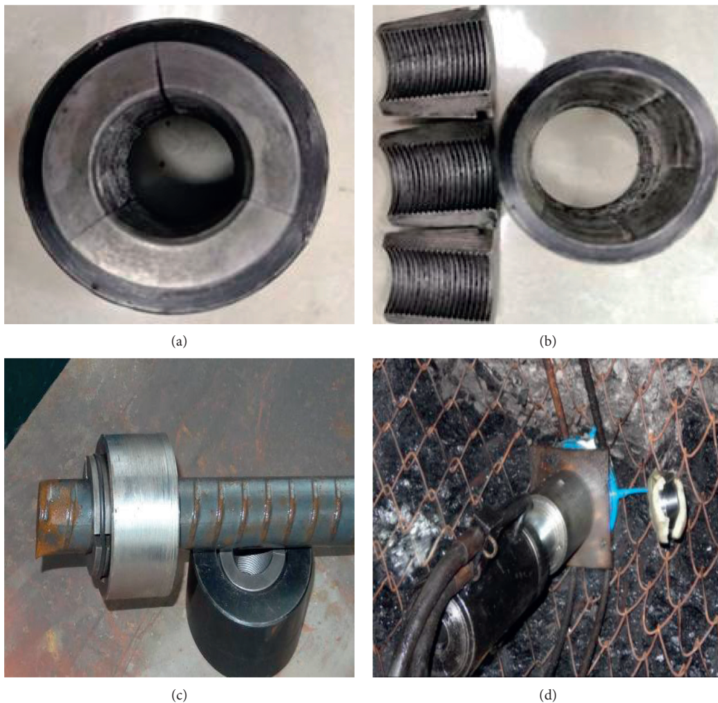
FIGURE 7: The anchoring system components: (a) barrel and wedge; (b) separated barrel and wedge; (c) barrel and wedge installed in the rock bolt; (d) barrel and wedge installation.
