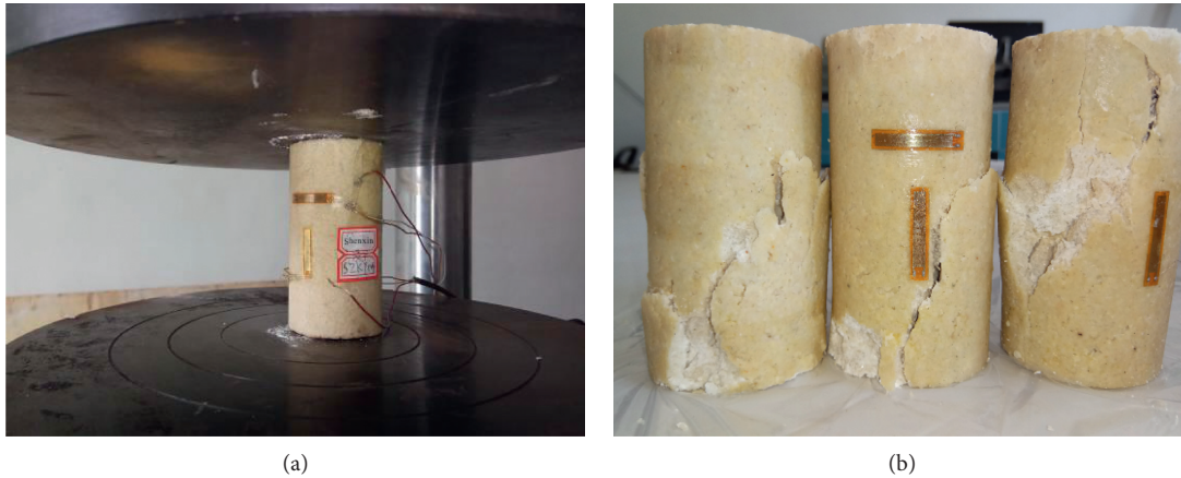
FIGURE 10: Process of uniaxial compression test and failure specimen. (a) Specimen installation. (b) Failure specimen.
