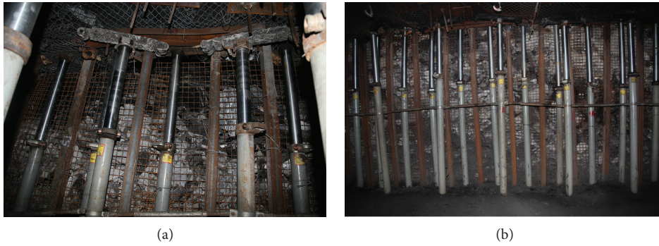
FIGURE 18: Gangue collapse process at 10 m footage: (a) behind working face 20 m; (b) behind working face 40 m.
