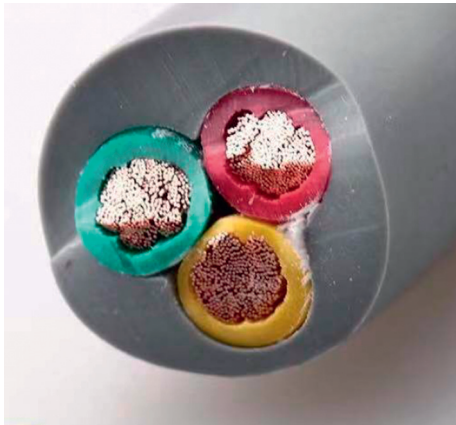
FIGURE 2: The image of the cable sample.
