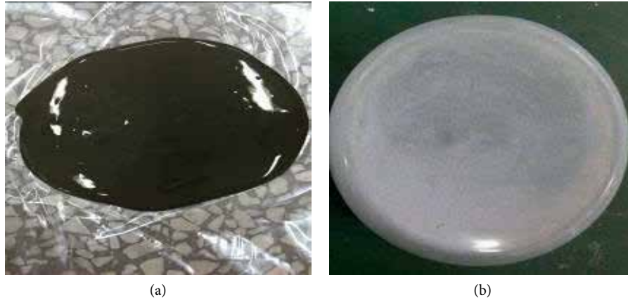
FIGURE 1: Photographs of the new solidified sealing material. (a) Flow condition. (b) Solidification state.
