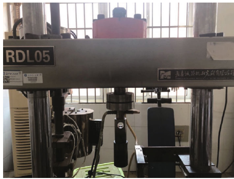
FIGURE 3: RDL05 testing machine of the tensile experiment. The maximum load of the machine is 50 kN.
