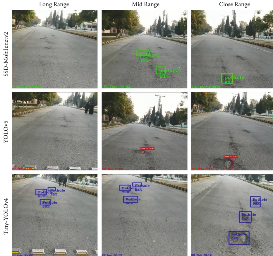
FIGURE 10: Real-time detection of potholes using OAK-D and Raspberry Pi on different distance ranges.
