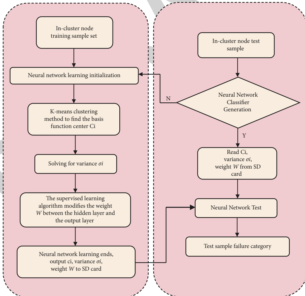
FIGURE 4: Cluster-head node feature-level fusion algorithm flow.
