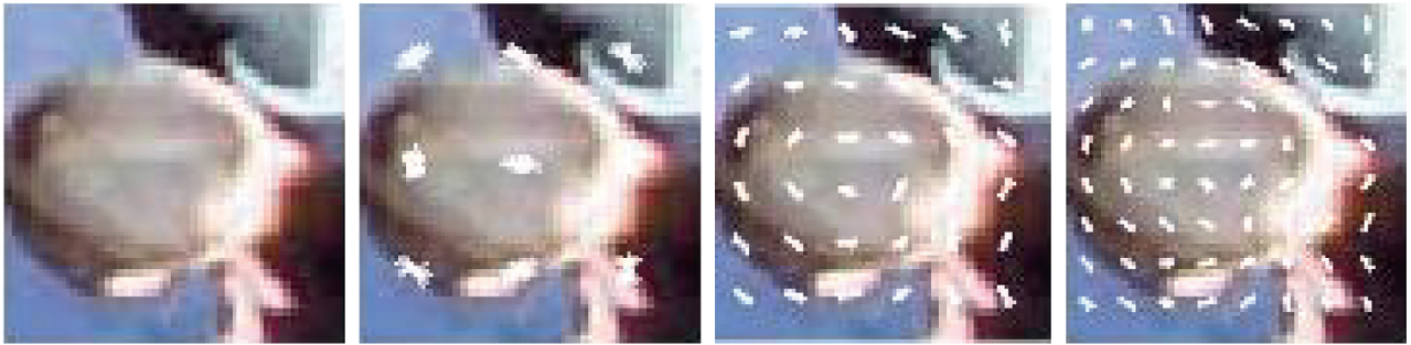
FIGURE 8: From left to right: the original object image [51, 51] px and images with highlighted gradients of HOG features for cell of sizes [16, 16] px, [8, 8] px, and [6, 6] px, respectively. The length of white abscissae is related to the gradients in the image.
