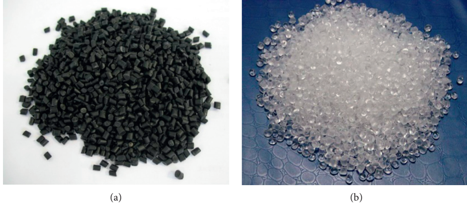
FIGURE 7: Blend components: (a) polypropylene (PP); (b) polyolefin elastomer (POE).
