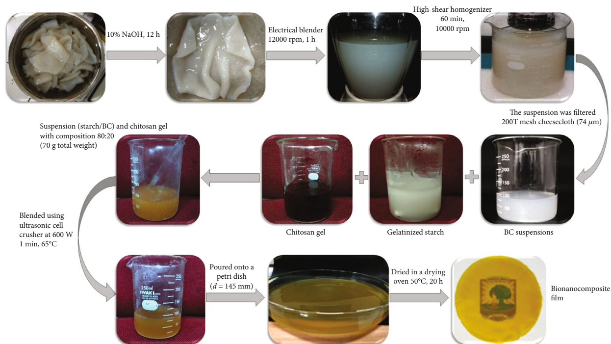
FIGURE 1: Steps of sample preparations for biocomposite.
