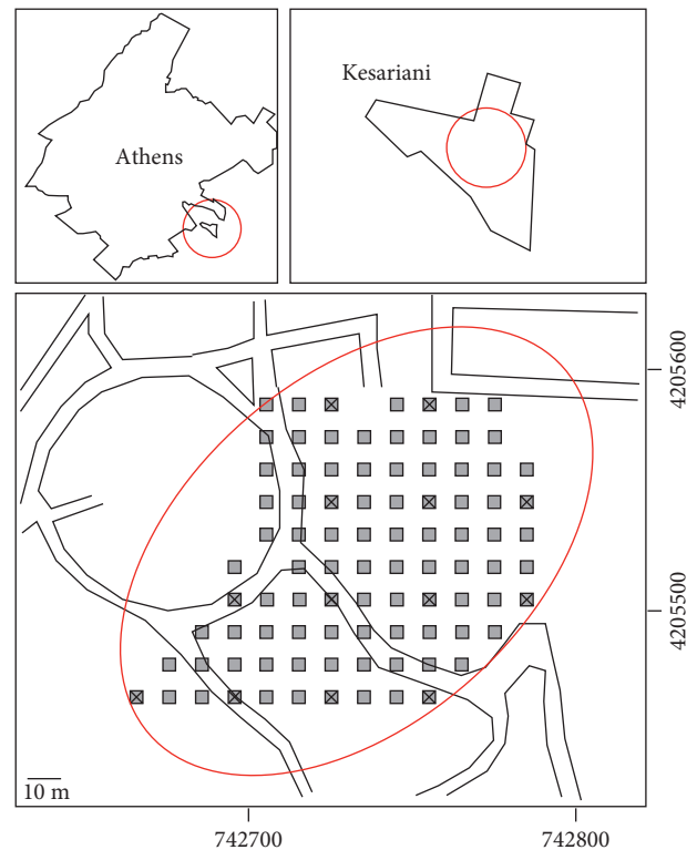
FIGURE 1: Sampling locations for Pb exposure analysis. Gray squares represent samples analyzed by using XRF only. Crossed grayed squares represent samples analyzed by XRF and ICP-MS.
